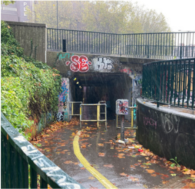
Impermeable ground surface means rain water run-off (and leaves in Autumn) are 'funnelled' into subway.
